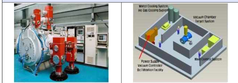
[그림4-16] High heat flux test facility with electron beam
